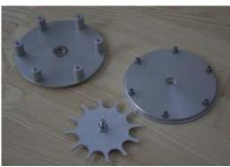
2. **Mount Pier Adapter top baseplate on TTS-160 Mounting Head**The altitude clutches on the Mounting Head is locked firmly. Place the Mounting Head on a stable table upside down on the Telescope Saddle plate.
