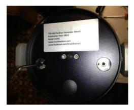
5. First loosen hexagonal socket screw behind each of the two plastic caps.
